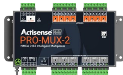
Figure 2 Actisense PRO-MUX-2 is a NMEA 0183 Multiplexer designed for marine environments. It enables combining data from up to eight NMEA 0183 talkers and routing them to six listeners, featuring advanced filtering, isolations on all inputs/outputs, and Ethernet configuration capabilities for complex vessel navigation networks. [23]
